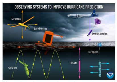
Schematic diagram illustrating 2022 hurricane observations by uncrewed underwater, surface, and aerial vehicles in conjunction with aircraft observations. Credit: Sarah Battle
