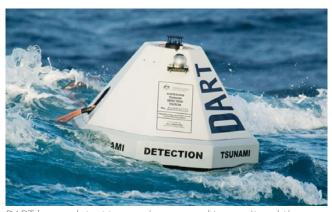
DART buoys detect tsunami waves and transmit real-time sea level information measurements back to the Tsunami Warning Centers. Credit: NOAA
