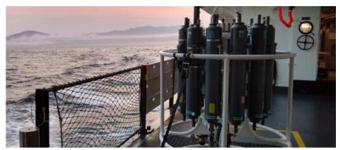
A conductivity, temperature, and depth instrument is shown on deck. Scientists gathered water samples at multiple depths across 186 locations off the West Coast during hake surveys on the NOAA Ship *Bell M. Shimada* in 2019. Photo credit: NOAA Fisheries
