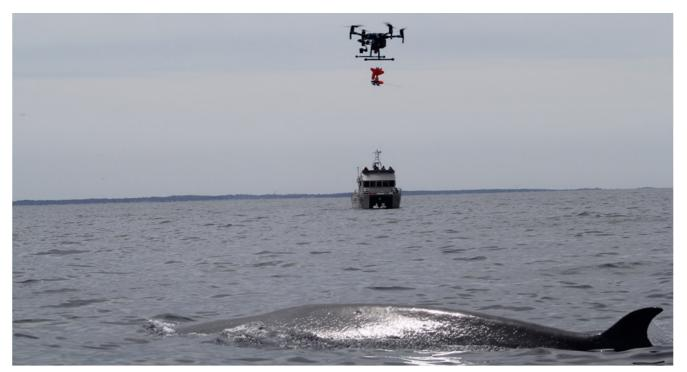
An uncrewed aerial system (UAS) attaches a suction-cup equipped synchronous motion, acoustic recording tag (DTAG) to a sei whale. This is the first time a UAS was used to tag sei whales and the first use of a UAS to tag free-swimming large whales in U.S. waters. Photo taken under NOAA Fisheries Permit No. 18786-06. Photo credit: Laura Howes
